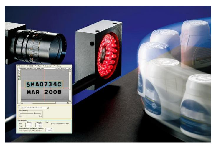
The System Offers Significant advantages over the Traditional Manual Human Inspection methods. While human inspectors working on assembly lines visually inspect parts to judge the quality of workmanship, machine vision systems use cameras and image processing software to perform similar inspections. Machine Vision inspection plays an important role in achieving 100% quality control in manufacturing, reducing costs and ensuring a high level of customer satisfaction.
